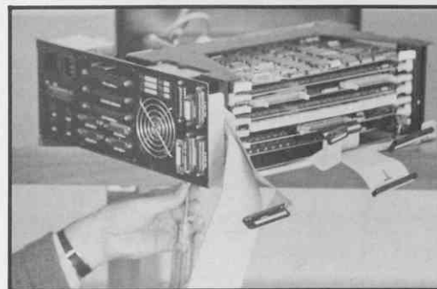
Figure 30 Screw Removal - Left Underside of Chassis
