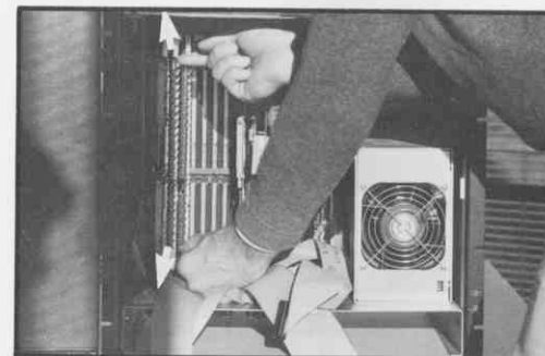
Figure 78 Removing the CPU Board
