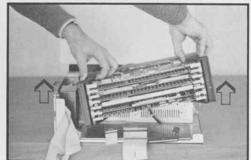
Figure 31 Card Cage Removal
